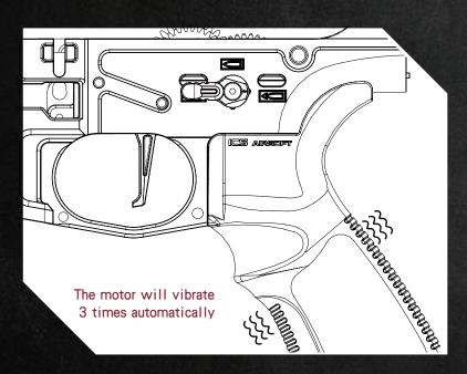
To avoid battery damage, the motor will stop functioning automatically after a short vibration if you continue using the product when the battery is depleted or low voltage.
